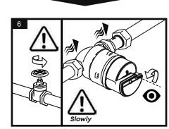
Turn on mains supply then valve slowly to bleed air / avoid over-speed damage to meter. Conduct leak check and check operation.
