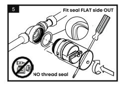
Fit new seal - stepped side in, flat side out. ↑ DO NOT use thread seal of any kind
