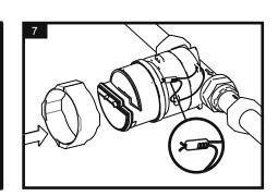
Fit tamper-evident security seal/s.
