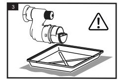
Prepare the work area by placing a drip tray and towel beneath the manifold to capture any water spillage.
