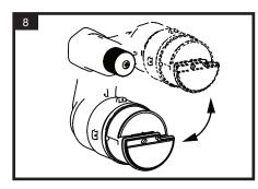
Turn the meter to the best reading position before tightening the locking nut and meter in place.
