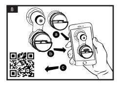
Photograph BOTH serial number with reading (meter face) and AMR number (side) of BOTH
