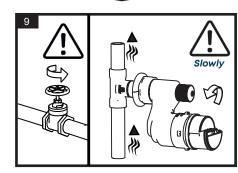
Turn on mains supply then valve slowly to bleed air / avoid over-speed damage to meter. Conduct leak check and check operation.
