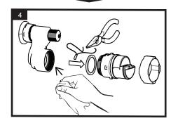
Remove old measuring capsule and seal/s. Clean the seat and gasket surfaces.
