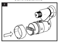
Fit tamper-evident security seal/s.
