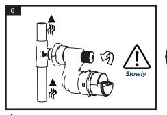
Turn on mains supply then valve slowly to bleed air / avoid over-speed damage to meter. Conduct leak check and check operation.
