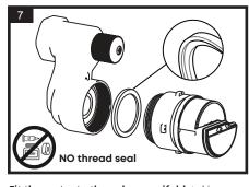
Fit the meter to the valve manifold, taking care that the stepped gasket is fitted as intended, and the O-ring on the capsule is in place and intact.
