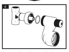
Place the **O-ring on the connecting piece**, fit to the manifold and lightly tighten onto the connector with the locking nut.
