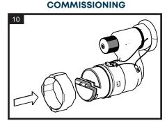
Fit tamper-evident security seal/s.
