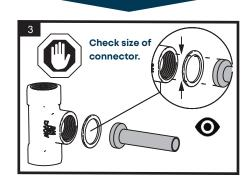
🕂 Check connector size is correct. i.e. Ensure that the seat on the fill tube fits the seat of the valve body.
