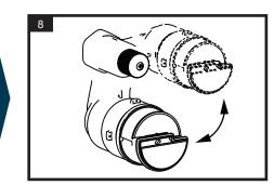
Turn the meter to the best reading position before tightening the locking nut and meter in place.
