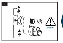
▲ Turn on mains supply then valve slowly to bleed air / avoid over-speed damage to meter.
