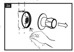
Remove and discard old valve. Clean the valve body, seat and gasket surfaces. Flush the line as needed.
