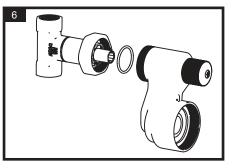
Place the O-ring on the connecting piece, fit to the manifold and lightly tighten onto the connector with the locking nut.
