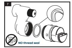
Fit the meter to the valve manifold, taking care that the stepped gasket is fitted as intended, and the O-ring on the capsule is in place and intact. \Lambda DO NOT use thread seal of any kind.
