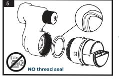
Fit the meter to the valve manifold, taking care that the stepped gasket is fitted as intended, and the O-ring on the meter is in place and intact. ① DO NOT use thread seal of any kind.
