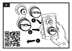
Photograph BOTH serial number with reading (meter face) and AMR number (side) of BOTH a) old capsule and b) replacement capsule, THEN c) scan QR Code to submit photos and details.
