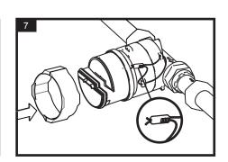
Fit tamper-evident security seal/s.
