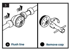
a) **Flush the line** to remove any debris.
