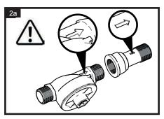
Apply thread seal to **male threads only**. Fit mini dual check valve to outlet.
