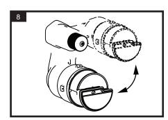
Turn the meter to the best reading position before tightening the locking nut and meter in place.
