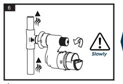
Turn on mains supply then valve slowly to bleed air / avoid over-speed damage to meter. Conduct leak check and check operation.
