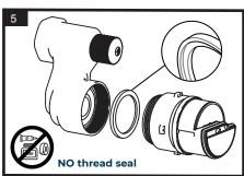
Fit the meter to the valve manifold, taking care that the stepped gasket is fitted as intended, and the O-ring on the meter is in place and intact.
