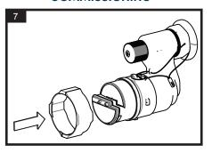
Fit tamper-evident security seal/s.
