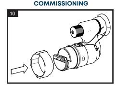
Fit tamper-evident security seal/s.
